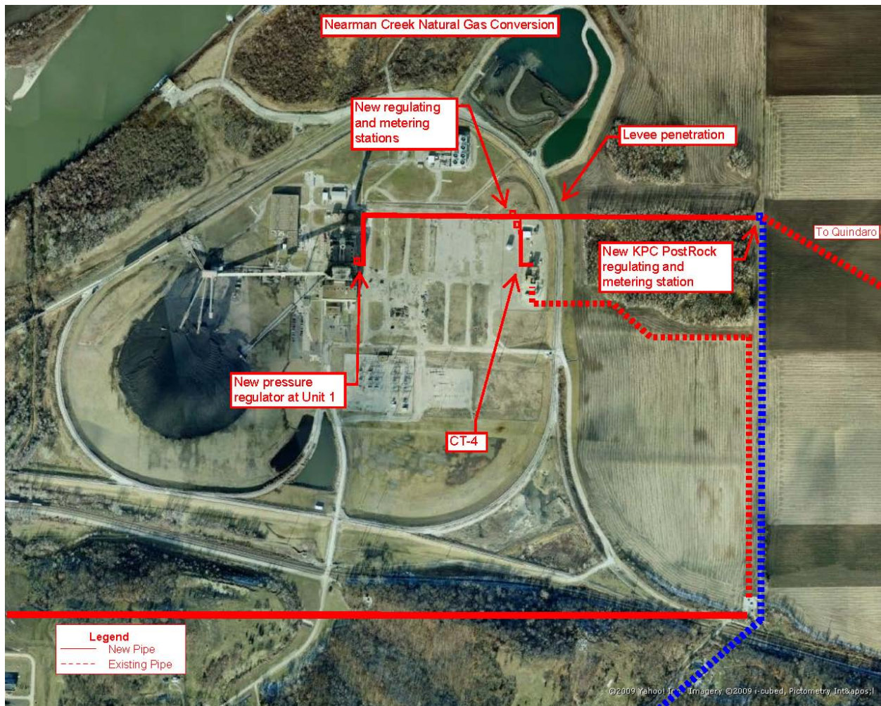
Figure 2-1 Gas Supply Pipeline Addition
